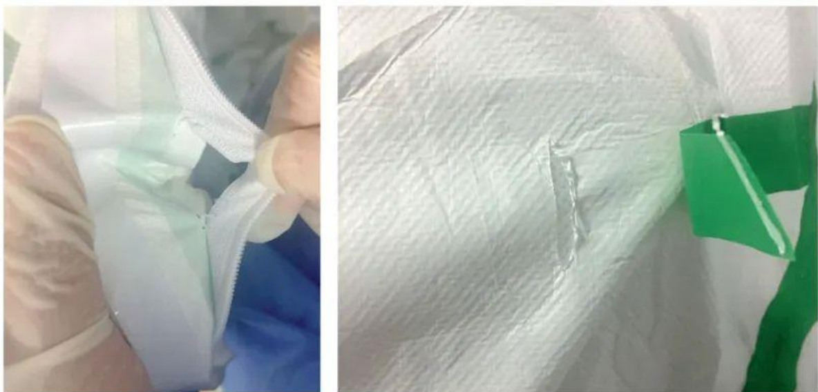
Figure 4-1 The protective clothing appeared to be stretched and damaged
